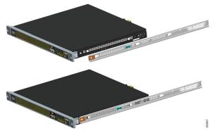
Use a Phillips screwdriver to secure the inner slide rail with one Phillips flat-head screw  $^{\textcircled{B}}$ .
